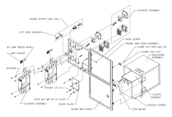
Turn off AC power. Unlock coin door and swing open. Unlatch and remove each coin mechanism separately to clean or replace with different type. Ensure mechanism seats fully in holder upon reinstallation. Close and lock release latch, then close door. Turn on game and change mechanism setup. Test known good and bad coins to verify operation.
