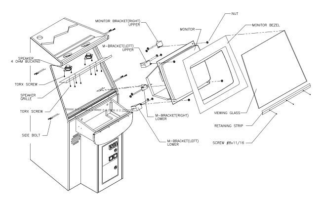
Remove viewing glass and bezel. Remove nuts holding monitor to brackets. Perform anode discharge.
