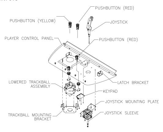
**BUTTONS.** Pry tab on bottom of button assembly to release switch. Unscrew plastic nut beneath control panel and remove button housing through top of control panel.
