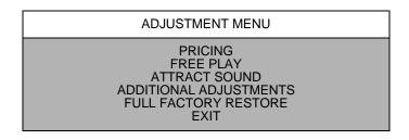
The Adjustments Menu offers several options. Press the Volume Up or Volume Down button to highlight an option and press the Test button. Each time an option on the menu is activated you are provided with multiple setting choices.
