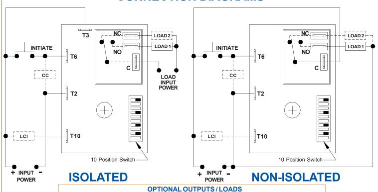
LOAD 2 = AUXILIARY LOAD (OFF DURING TIMING) CC = COIN COUNTER
